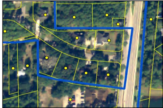
Figure 6. Parcel centroids (yellow points) used in summarizing parcels (yellow) to utility service area boundaries (blue)
